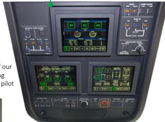
(above) Korry's world-first utility control system with integrated touchscreen controls for the Gulfstream G500/G600/G700 aircraft
