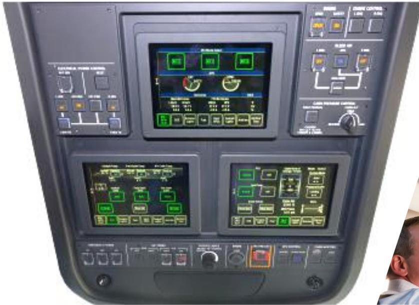
The world's first touchscreen overhead control panel developed and produced by Korry for the Gulfstream G500/600
